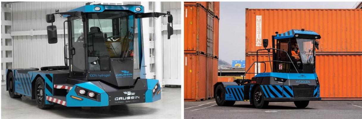
*The ATM®-H2 (left) and the APM®-H2 (right), two emblematic GAUSSIN hydrogen vehicles*
