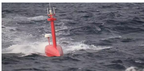
DriX autonomous drone in operation at sea force 5
